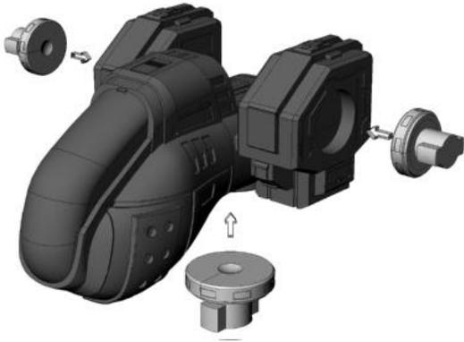
3. Glue the male half of the ¾ inch Plug and Twist joint to the bottom of the Main Hull.
