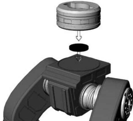
2. Place the Large O-Ring into the joint.
